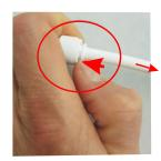
Remove the blue c-ring. Hold the elbow as shown below. Press nail toward the elbow. The same time use another hand to pull tubing out.
