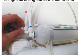
Use fingers or collet tool to disconnect tubing (fourth stage). Push on top of fitting, pull tubing out at the same time
