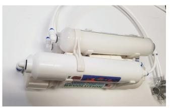
Remove blue c-rings from elbow on stage
