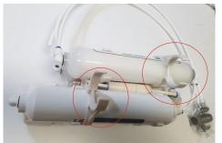
Cut tubing piece 13 ½". Make sure to cut under 90 degrees.
