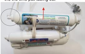
Use fingers or collet tool to disconnect tubing (fifth stage). Push on top of fitting, pull tubing out at the same time
