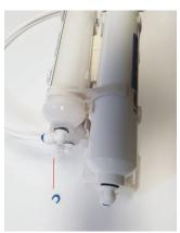
Use fingers or collet tool to disconnect tubing (fourth stage). Push on the top of fitting, pull tubing out at the same time
